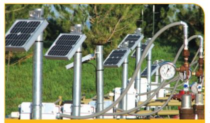
**Sophisticated monitoring:** demonstrating photovoltaic solar panels transmitting well data. **Photo:** Richard Ranger
